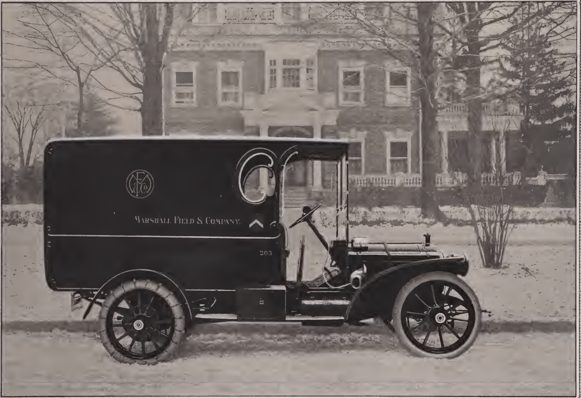
Fast light delivery body fitted to used Packard chassis
